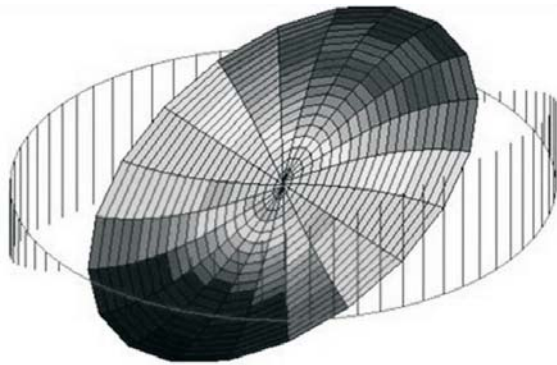
Fig. 5. Contour plot of simulated B_r and B_z with a current 1.0A of mode 11.
