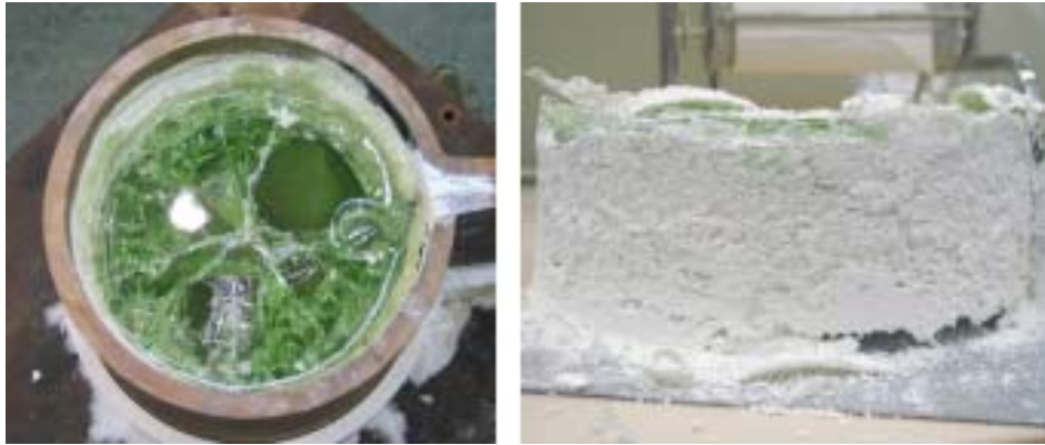
Fig. 5. Solidified ingot of glass in the inductor crucible (left) and after removal from the inductor crucible (right).
