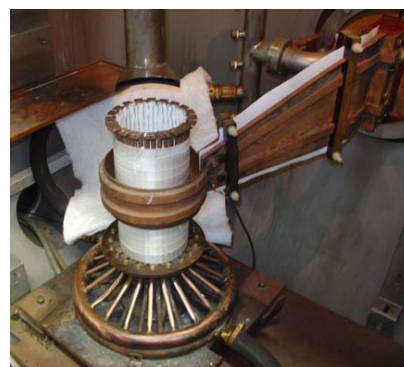
Fig. 2. Cold crucible and inductor.
